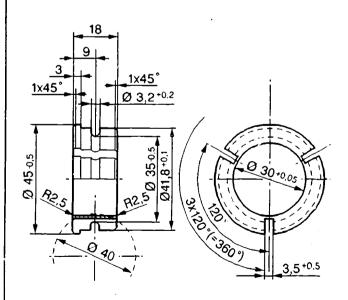
Pressing-in mandrel for cylindrical roller bearing in drive/reduction gear end shield:
